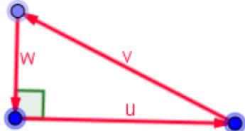
$$\begin{aligned} w+u &= v \\ v \cdot v &= |v|^2 \cdot \cos 0^\circ = |v|^2 \\ u \cdot w &= 0 \quad (\text{perpendiculares}) \end{aligned}$$
