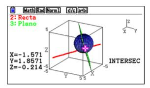
The projection point has coordinates  $P\left(\frac{-11}{7}, \frac{13}{7}, \frac{-3}{14}\right)$ . We calculate the square of the distance between the center O and the projection P.
