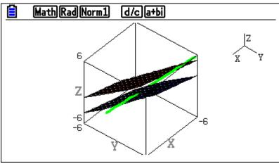
Whit the function G-Solv, determine the intersection of the line and each of the planes.
