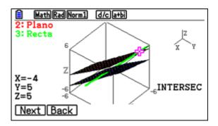
The coordinates of the intersection point of the plane  $\Pi \equiv x + 2y - 2z - 2 = 0$  and the straight
