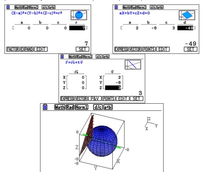
We determine with the function *G-Solv*, the intersection of the line and the plane:
