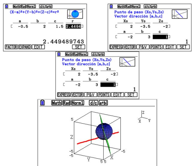
Whit the function G-Solv, determine the intersection of the line and the plane (projection point)
