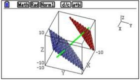
To determine the intersection of the plane  $\Omega \equiv 6x - 3y - 2z + 63 = 0$  and the straight  $r \equiv (x, y, z) = (5, -1, -1) + \alpha(6, -3, -2)$  function *G-Solv* is used:
